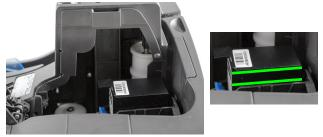
• The cartridge should appear parallel with the top of the ink cartridge platform when seated. Close the cover and secure into place by pressing down on the indent marks.
